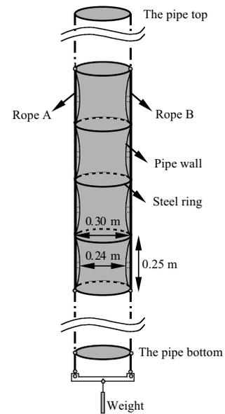
Fig. 2. Diagram of the pipe employed in the Mariana experiment.
