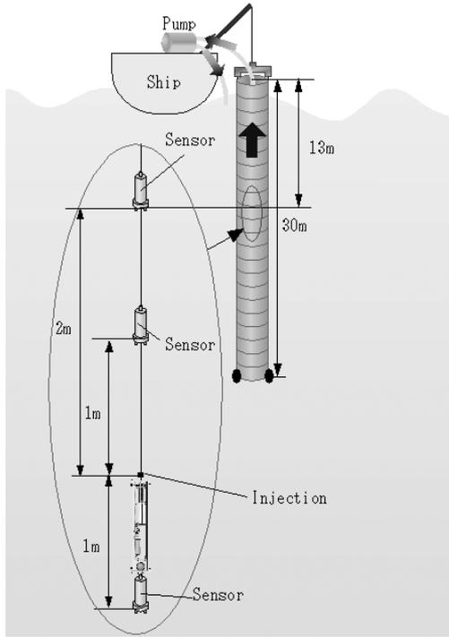
Fig. 7. Diagram of experimental apparatus (Onagawa Bay, Japan, September, 2003).
