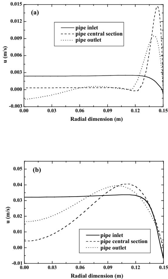
Fig. 9. Upwelling velocities inside the pipe under steady-state flow condition. (a) thermal diffusivity  $a = 10^{-9} \text{ m}^2/\text{s}$ ; (b) thermal diffusivity  $a = 10^{-5} \text{ m}^2/\text{s}$ .
