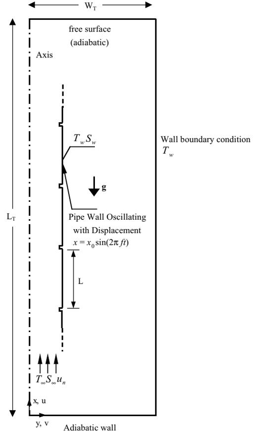
Fig. 3. Baffled pipe geometry with coordinate system.
