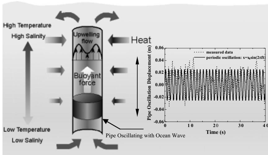
Fig. 1. Conceptual principle of the perpetual salt fountain. Right panel shows variations of pipe oscillation displacement with time. Pipe motion is simplified as a periodic oscillation, in which the oscillation amplitude and frequency represent the average values of the amplitudes and frequencies of the pipe motion.
