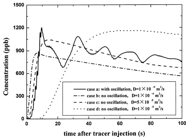
Fig. 5. Relation between elapsed time from tracer injection and its concentration.
