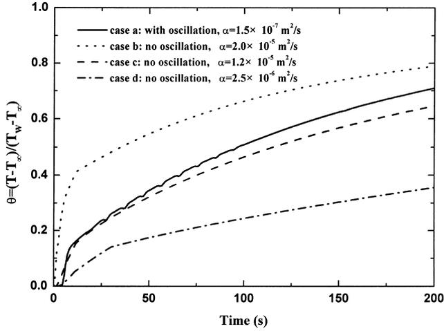
Fig. 6. Relation between elapsed time and computed temperature.  $\theta$  is dimensionless temperature, and  $T_w$  and  $T_\infty$  are wall temperature and ambient water temperature.
