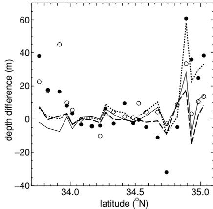
Fig. 5. Difference of depths (in meters) between the gridded topography data and the ADCP beam along the ferry line. Black and white circles indicate the DBDB-V and ETOPO-2, dotted, dashed, and solid curves correspond to the SKKU, JTOPO1, and an optimal combination E1, respectively. The rms differences between the data sets and the beam depths are 21.0, 12.7, 15.4, 6.6, and 8.4 m for the DBDB-V, ETOPO-2, SKKU, JTOPO1, and the estimates E1, respectively.
