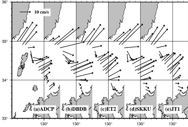
Fig. 2. Mean barotropic velocity distribution by (a) ADCP measurement and by (b)–(e) numerical experiments with several bottom topographies. The averages were taken over 5-year winter and over depth. The model results are shifted to the east by  $1^\circ$ , respectively.
