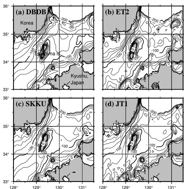
Fig. 1. Bottom topographies of the Tsushima/Korea Straits based on (a) DBDB-V, (b) ETOPO-2, (c) SKKU, and (d) JTOPO1.
