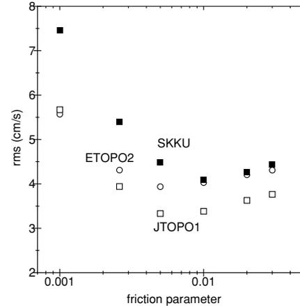
Fig. 3. RMS velocity differences of the simulation and the ADCP measurement as a function of the friction parameter  $r$ . The open circles, closed and open squares indicate the experiments with the ETOPO-2, SKKU, and JTOPO1, respectively.
