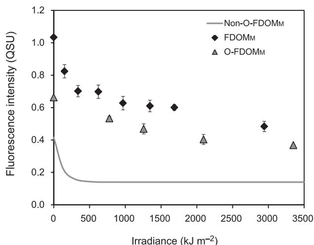
Fig. 3. Changes in the fluorescence intensity of  $FDOM_M$ ,  $O-FDOM_M$  and non- $O-FDOM_M$  in sunlight irradiation experiments. The fluorescence intensity of non- $O-FDOM_M$  was estimated by subtracting the intensity of  $O-FDOM_M$  from that of  $FDOM_M$ . Error bars of  $FDOM_M$  and  $O-FDOM_M$  represent standard deviations ( $n = 3$ ) and ranges ( $n = 2$ ), respectively.
