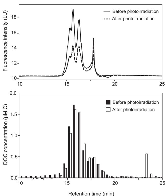
Fig. 5. Size exclusion chromatograms of a) O-FDOM<sub>M</sub> and b) O-DOC in sunlight irradiation experiments.
