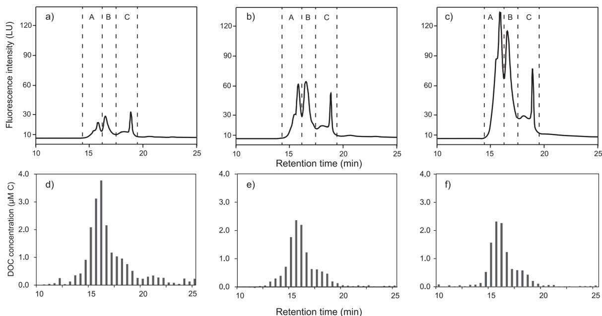
Fig. 1. Size exclusion chromatograms of O-FDOM<sub>M</sub> (a–c) and O-DOC concentrations (d–f) at 10 m (a, d), 150 m (b, e) and 1000 m (c, f).
