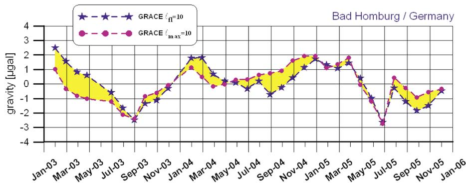
Fig. 6. GRACE-derived gravity variation filtered with a simple truncation ( $\ell_{\max} = 10$ ) and Gaussian filtering ( $\ell_f = 10$ ) of the spherical harmonic coefficients at BH in Germany from February 2003 to December 2005.
