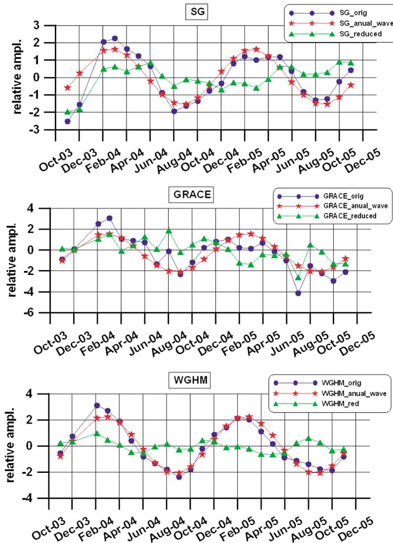
Fig. 11. Original data, annual wave, and reduced data (after subtracting the annual signal) for SG, GRACE, and WGHM at the BH site from November 2003 to October 2006.
