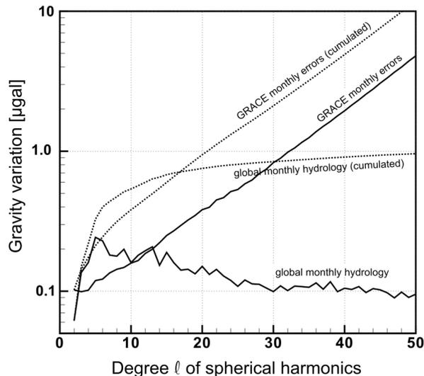
Fig. 1. Calibrated errors of the GRACE monthly solutions and gravity variations derived from the hydrology model (WGHM) (Döll *et al.*, 2003) as functions of degree  $\ell$  of spherical harmonics. Errors of monthly solutions per degree (solid line) and as function of maximum degree (dotted) are shown.
