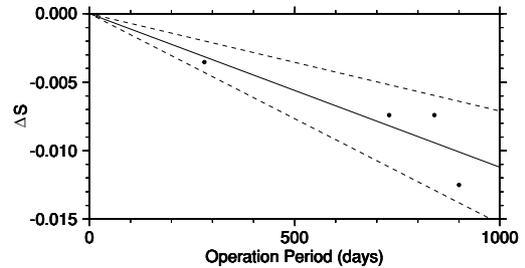
Fig. 5. Plots of the mean residual in equivalent salinity for the first post-recovery calibration ( $\Delta S$ ) against the operating period for Floats 1, 4, 5, and 6. The solid and dashed lines indicate the regression line through the origin and its 95% confidence interval.
