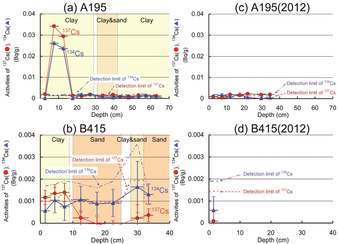
Fig. 2. Activities of  $^{137}\text{Cs}$  and  $^{134}\text{Cs}$  in core sediments sampled in October 2011 at (a) A195 and (b) B415 and in February 2012 at (c) A195 and (d) B415. The vertical error bars indicate counting statistic error ( $1\sigma$ ), and the detection limit is calculated as  $3\sigma$ .
