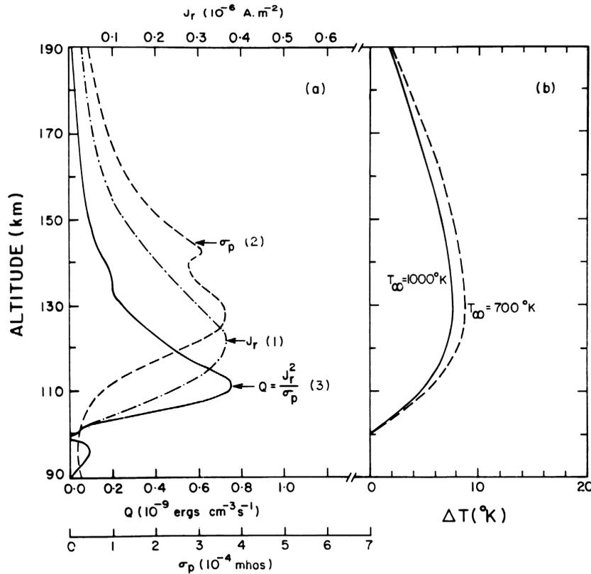
Fig. 1. (a): Altitude profile of (1) the vertical ion currents ( $J_r$ ), (2) the Pedersen conductivity  $\sigma_p$  and (3) the dissipated power due to Joule heating ( $Q$ ) over the dip equator for maximum east-west current density ( $J_\phi$ ) of  $10.4 \text{ Amp/km}^2$  at a local time of 1100 hrs. (b): The profile of the increase in neutral temperature due to Joule heating for two exospheric temperatures.
