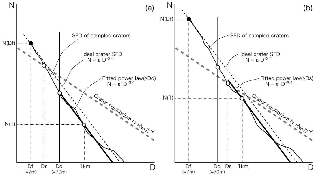
Fig. 1. Schematic representation of crater SFD measurement. Relative age is obtained by fitting the population SFD,  $N(D) = \alpha D^{-3.4}$  to SFD of craters  $\geq D_m$ . (a)  $D_d \geq D_s$ . Craters  $\geq D_d$  are used for SFD measurement (i.e.,  $D_m = D_d$ ). (b)  $D_d < D_s$ . We use  $D_m = D_s$ .
