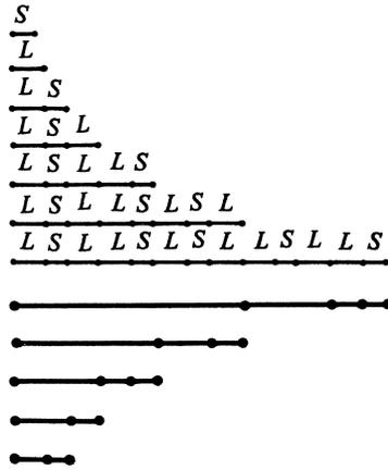
Fig. 1. One-dimensional quasicrystal and its self-similarity. The upper seven lines show the generating process of the Fibonacci sequence:  $L/S = (1 + \sqrt{5})/2$ . The lower five lines demonstrate self-similarity of the one-dimensional quasicrystal.
