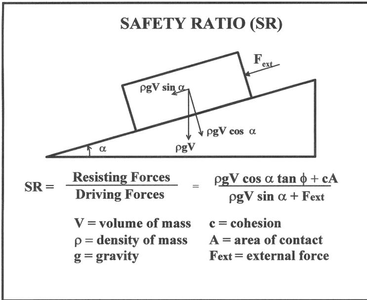
Fig. 3. Safety Ratio. Shows the geometry and forces of a free-body object resting on a solid surface.
