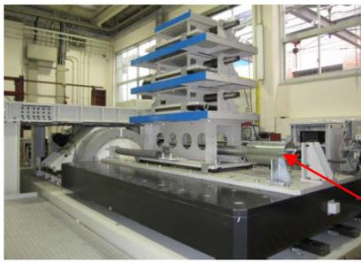
Magnetorheological rotary inertia mass damper
