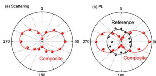
**Fig. 3** Polar plots of (a) dark-field scattering and (b) PL intensities of nanocomposites (red) and ensemble Si-QDs without Au nanorod (black) as a function of polarization angles. Reproduced with permission from *H. Sugimoto, et al., ACS Photonics, 2, 1298–1305 (2015)*. Copyright 2015, American Chemical Society.
