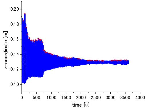
**Fig. 6** Numerically obtained time trace of particle position in  $z$ -component ( $Re = 10$ ,  $d_p = 8$  mm,  $\rho_p = 1200$  kg/m<sup>3</sup>)
