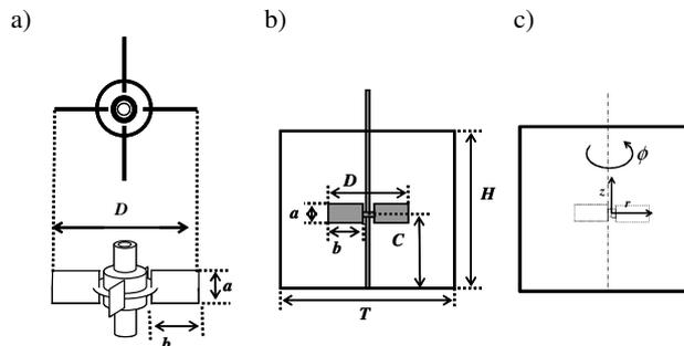
Fig. 1 Schematic of stirred vessel: a) turbine impeller, b) stirred vessel and c) coordinate system
