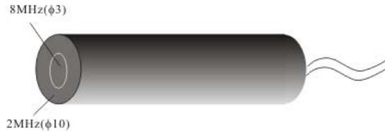
Fig. 3 Schematic of multi-wave transducer.
